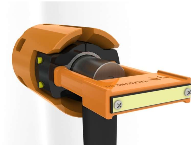
Figure 18: Yellow latching indicator buttons popped out (fully mated) on a Mk III or Mk IV connector
