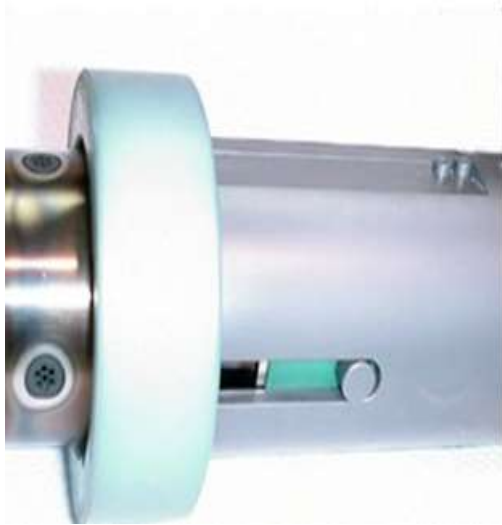
Figure 15: ROV Latch Fingers in the Closed Position (Mk II)
