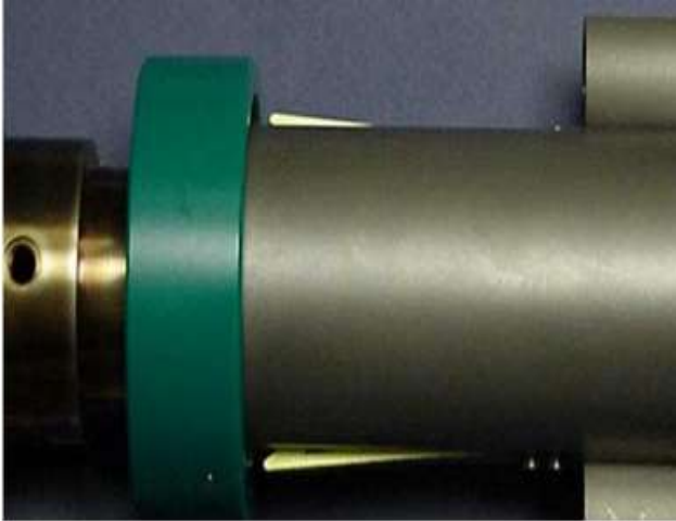
Figure 16: ROV Latch Fingers in the Open Position (Mk II)
