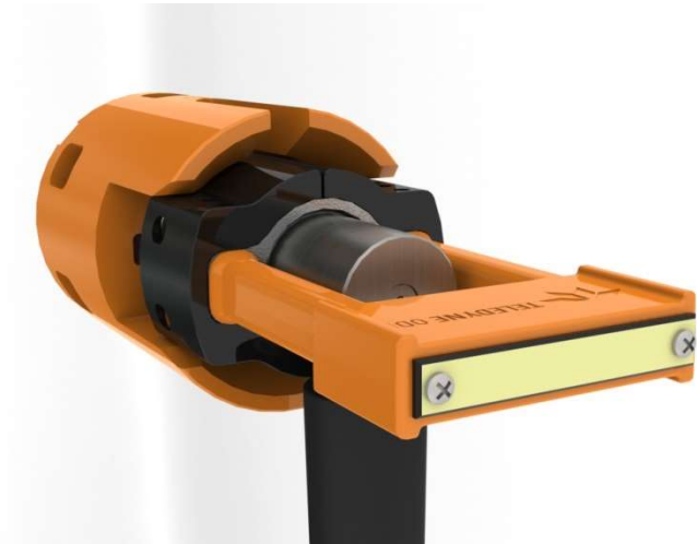
Figure 17: Yellow latching indicator buttons not popped out (not mated) on a Mk III or Mk IV connector
